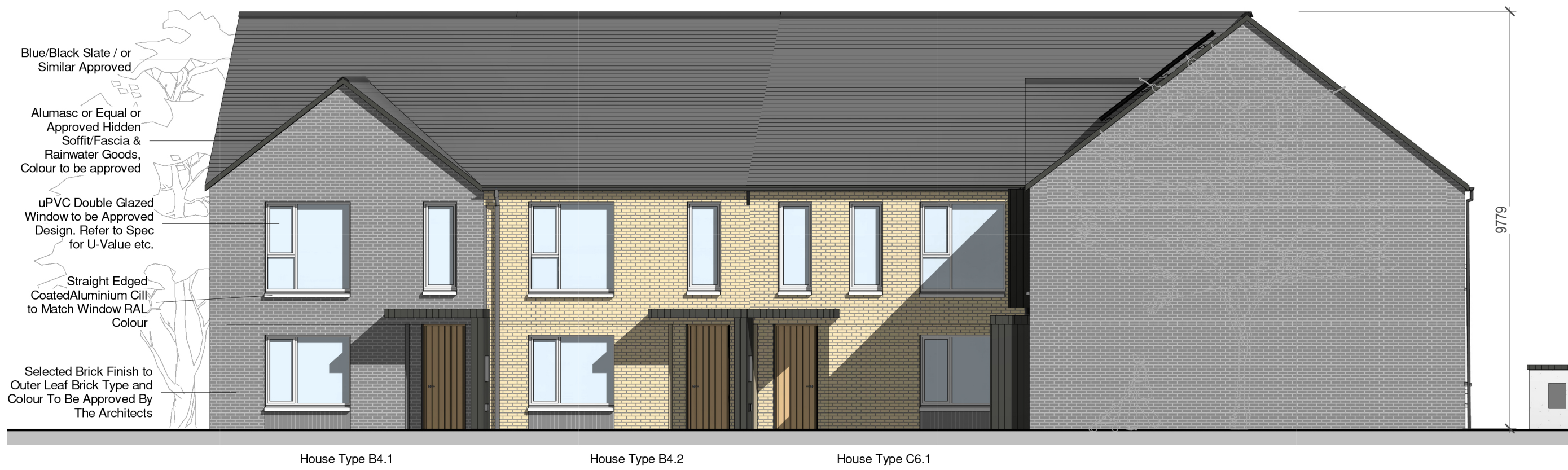
2 Block 6 - Front Elevation 2 1 : 100
